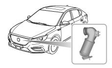
The exhaust system incorporates a catalytic converter, which converts poisonous exhaust emissions from the engine into environmentally less harmful gases. Catalytic
