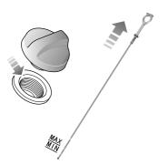
Check the oil level weekly and top up with oil when necessary. Ideally, the oil level should be checked with the engine cold and the car resting on level ground. However, if the engine is running and already getting warm, wait for at least five minutes after switching off the ignition switch before checking the level.
