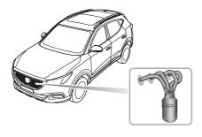
The exhaust system incorporates a catalytic converter, which converts poisonous exhaust emissions from the engine into environmentally less harmful gases.
