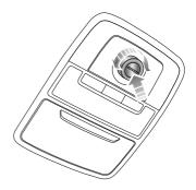
When the ignition switch is set to ACC or ON/RUN/START, you can operate the sunroof.
