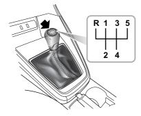
The manual transmission is a 5-speed transmission with 6 gears, which are: 1st, 2nd, 3rd, 4th, 5th, R (Reverse) respectively.
