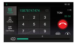
During a call, rotate the volume adjustment knob or press the volume adjustment button in the steering wheel controls to adjust the in-call volume.
