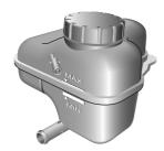
The coolant level should be checked weekly when the cooling system is cold and with the car resting on level ground.
