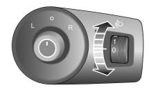
Position 0 is the initial position of the headlamp levelling adjustment switch. The headlamp levelling adjustment can be made as the following table according to the vehicle load.
