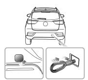
Your vehicle is equipped with towing holes at the front and rear, which are used for fitting the towing eye in the tool box. The tool box is placed in the spare wheel under the trunk floor. To fit the front towing eye, remove the small cover on the bumper, then screw the towing eye into the threaded hole in the bumper beam through the small hole (as shown in the figure). Ensure the towing eye is fully tightened.
