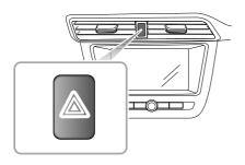
Note: When you have to stop or slow down the vehicle due to some emergent problems, always press the hazard warning lamp switch. And all the turning signal lamps and direction indicator lamps shall flash at the meantime to warn other road users.
