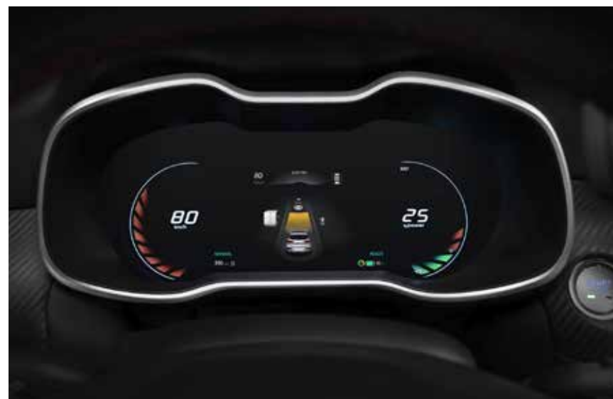
FULL DIGITAL CLUSTER WITH 7 inches EMBEDDED LCD SCREEN
